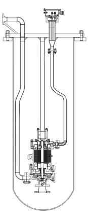
+ V Totally submerged solution ✓ Without long shaft line ✓ Low NPSHa application
