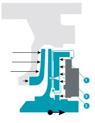
In the real functioning position, pressure in the chamber is regulated between high and low pressure. Resultant force is null and the mobile is stable and perfectly balanced between both.
